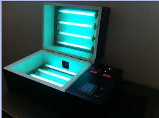
U V EXPOSURE UNIT 15W x 4 nos. UV exposure unit Auto timer
