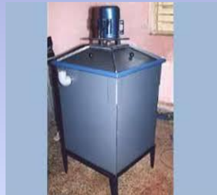
ETCHING MACHINE with corrosion free Chemical pump Temperature controlled heating
